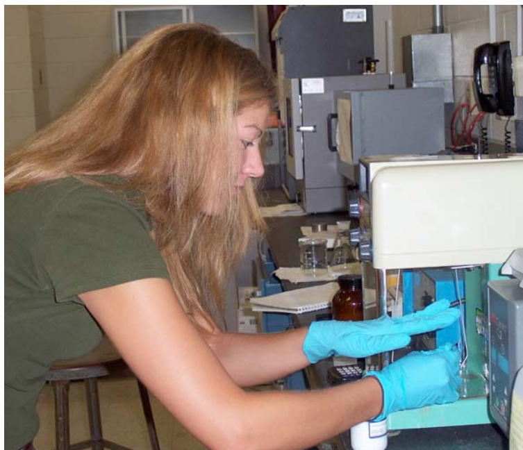
DREAMer Melissa Schillo uses a balance to weigh chemicals for her work on the synthesis of nanocrystalline semiconductor CdS particles (quantum dots) in DREAM Mentor Dr. Wei-Heng Shih's lab. Melissa's work was included in a patent filed in May 2005 entitled, SYNTHESIS OF WATER SOLUBLE NANOCRYSTALLINE QUANTUM DOTS AND USES THEREOF.
